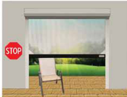
Obstacle will be detected and motor stops running.
